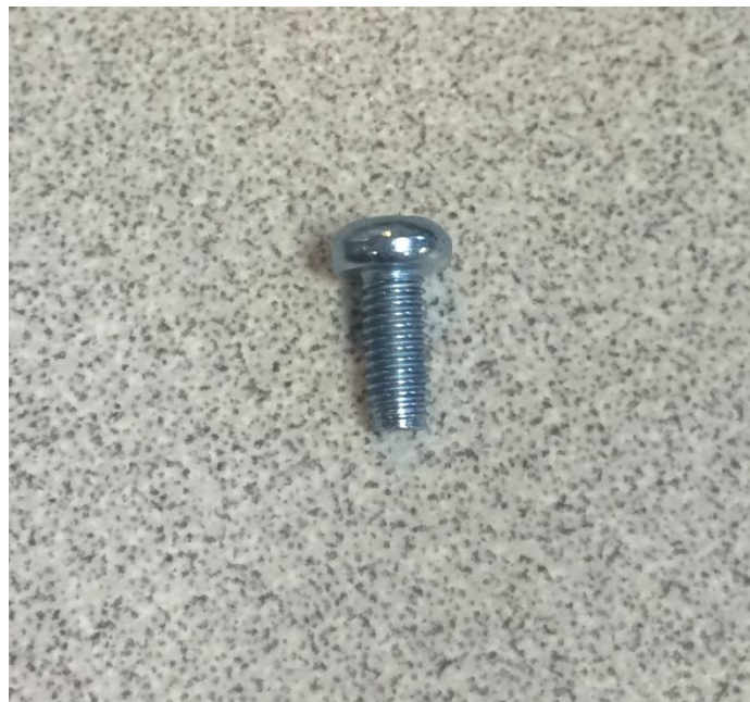
Figure 1: Taptite II M3.0 x 0.5 x 7mm Torx® Pan Head with T10 Torx® Recess
