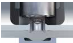
Step 2 Creating centre cut-off and welding
